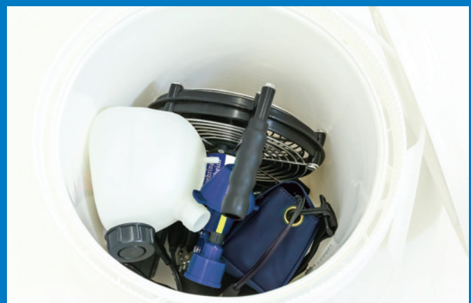
The spinning atomizer disc and the fan disperse the vaccine into the air. This helps to ensure an even vaccine distribution to all of the birds. They can easily be removed to clean.
